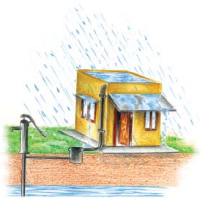
(a) Recharge through Hand Pump
